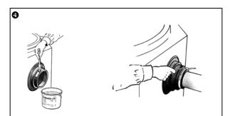
Lubricate with a thin coat of Forsheda Lub over the rubber part. Connect the pipe and fit the clamping band in place. Tighten the screw so that the rubber is compressed against the connecting pipe.
