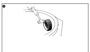
Place the seal in the hole and tap it into the correct position using a rubber or plastic mallet. Tap the end of the short plastic supporting ring that is fitted in the seal.
