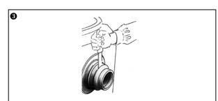
Decide which size collar is appropriate for the connecting pipe. Cut away the surplus part of the coupling using a knife. A special recess is provided for this purpose.
