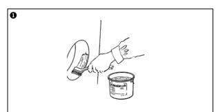
Lubricate the drilled or prefabricated hole using Forsheda 992 Lub.
